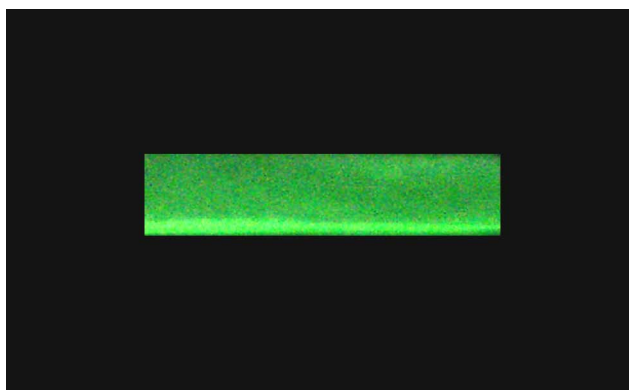
Figure 1. Green luminescent Tb 3+ :PVA polymer film under a UV lamp.
